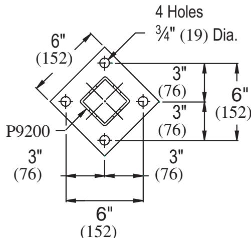
Standard Dimensions for 1 5/8" (41mm) width series channel fittings (Unless Otherwise Shown on Drawing)
