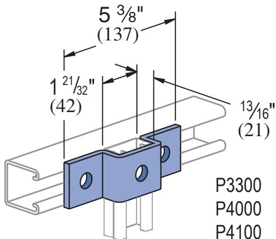
Standard Dimensions for 1½" (41mm) width series channel fittings (Unless Otherwise Shown on Drawing)
