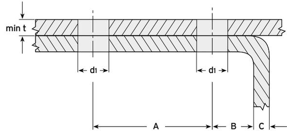
► Sizes 5/8" and 3/4" require outer ply thickness (min t) to be at least 5/16".
