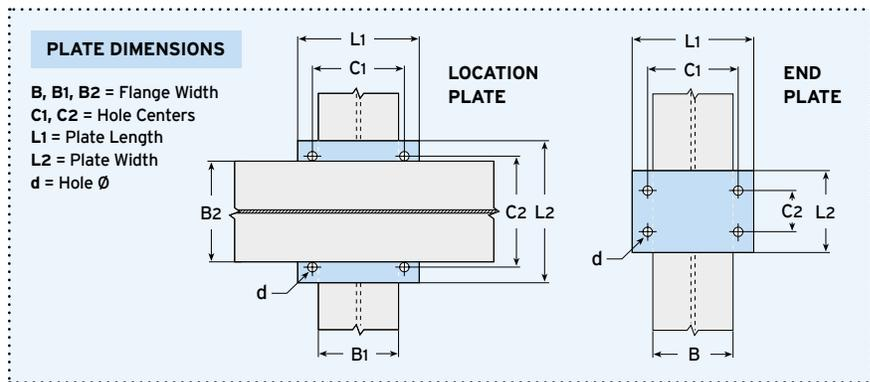
Material: Structural steel grade A572 Grade 50. For other grades contact Lindapter.
