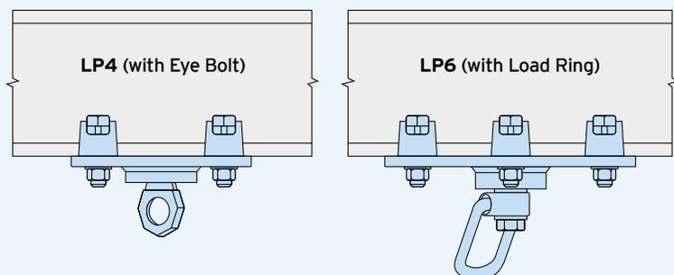
\* The Type LP safe working load is limited to the capacity stamped on the load ring/eye bolt.
