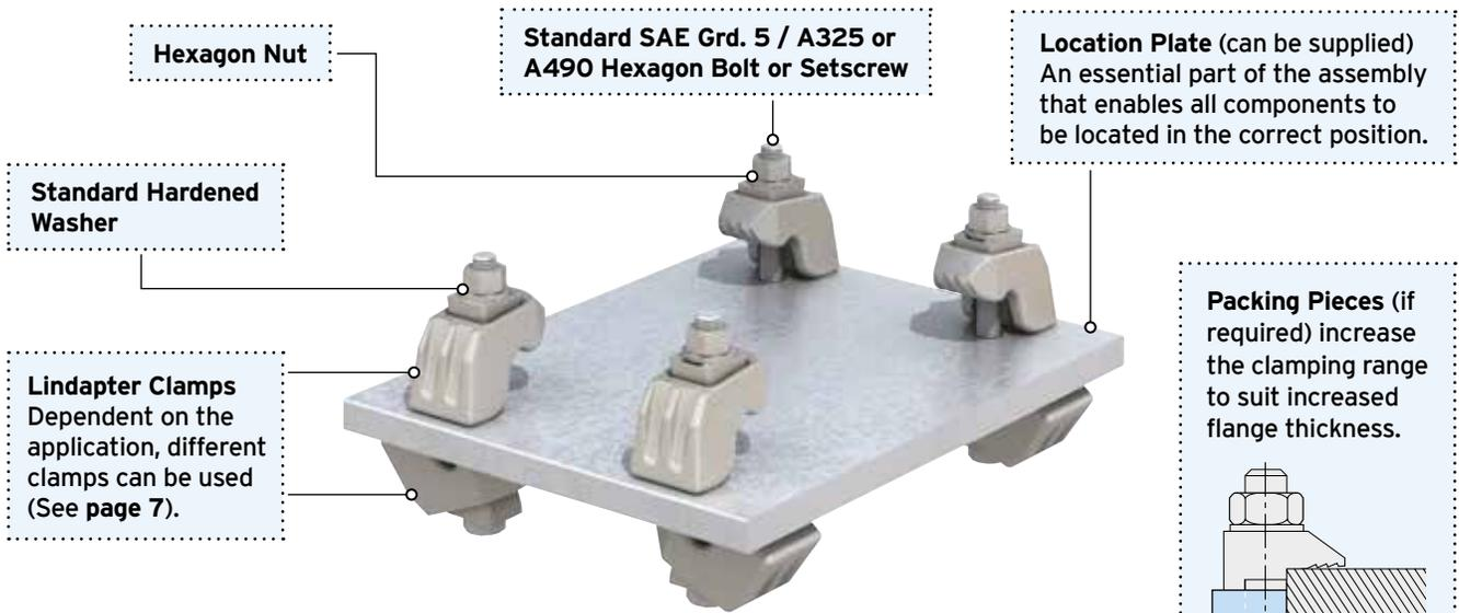
This example is configured with Lindapter AAF clamps (code LAAF075) and four A490 bolts.
