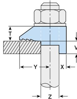
Material: Malleable iron, zinc plated / hot dip galvanized.
