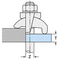
Mild steel, malleable iron, zinc plated / hot dip galvanized.
