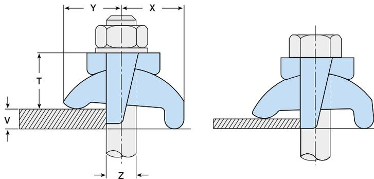
Note 1: When installing, ensure the straight (not tapered) leg of the saddle is in contact with the flange.
