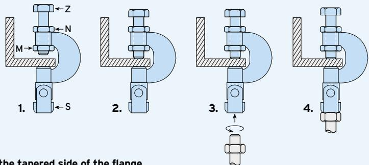
➤ Ensure that the cup point setscrew always grips on the tapered side of the flange.
