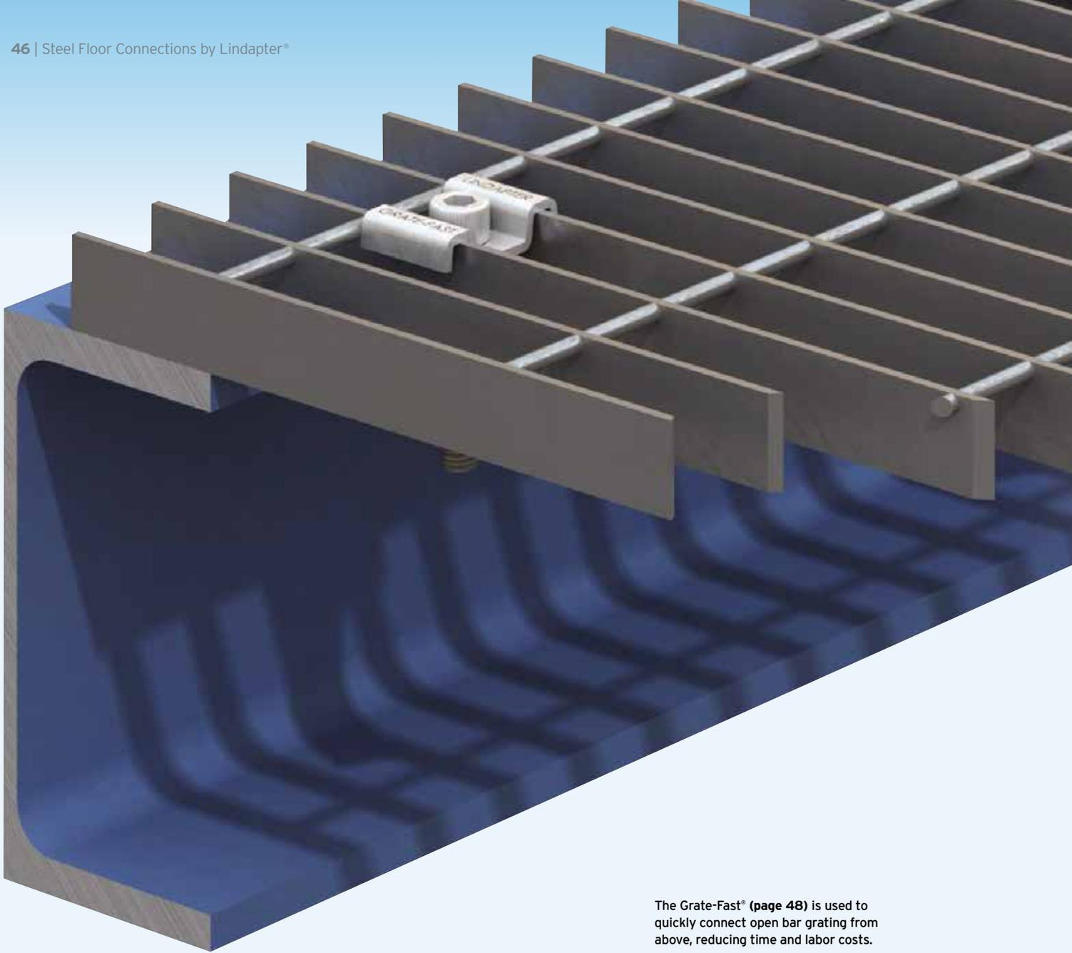
The Grate-Fast® (page 48) is used to quickly connect open bar grating from above, reducing time and labor costs.
