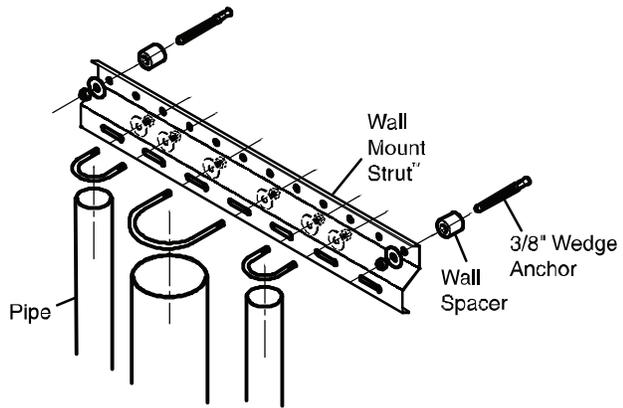
Wall Mount Strut® is made of heavy-duty 12 ga. 304/316 stainless steel and is available in precut lengths of: 12", 24" 48" and 120".
