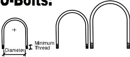
Food Grade Strut(R) U-bolts are fabricated to accommodate trade sizes of conduit and tubing. Each U-bolt has minimum thread to ease assembly and minimize exposed threads.
