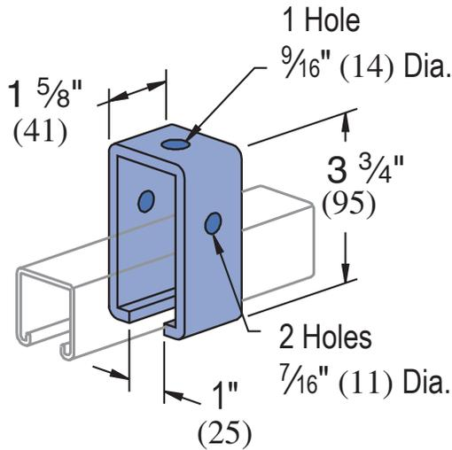
**Standard Dimensions for 1 5/8" (41mm) width series channel fittings (Unless Otherwise Shown on Drawing)**
