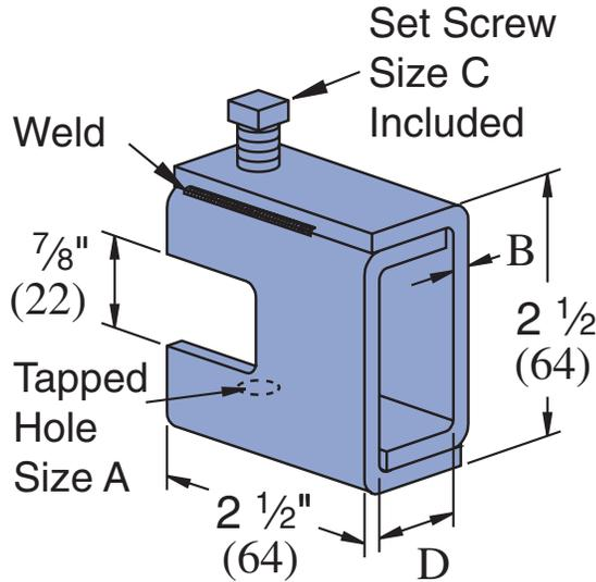
Weld is not continuous it is either 1 1/4" (32) - 1 3/4" (45) long or 2 spot welds. All welds are on the top and bottom.
